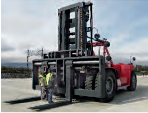
Fork positioners - load capacity 55,000 kg / 1,200 mm
