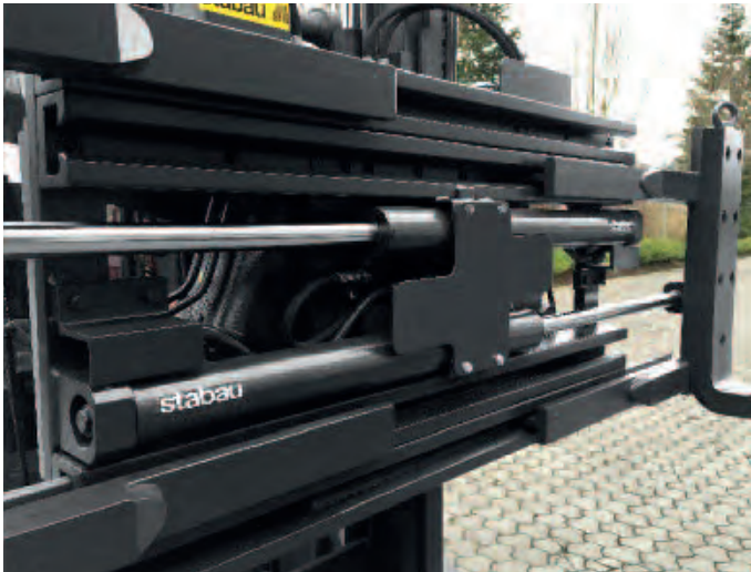
Bumpers for the hydraulic connection of cylinders optionally available
