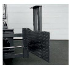
Clamp arm with additional load-securing device
