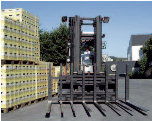
Handling of 8 pallets with empties or 6 pallets with full products. Lift truck: 8,0 to/900 mm LC or 9,0 - 10,0 to/600 mm LC
